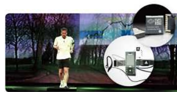
VTI’s SOI-MEMS multi-axis accelerometer is the “stride sensor chip” in the miCoach real-time training system (Courtesy: VTI Technologies, adidas and Samsung)
