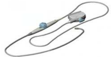
Transesophageal probes, which are inserted into the esophagus via the throat, send a beam across the esophageal wall to image the heart structures. The constraints on space and power consumption for the embedded electronics are extremely stringent.
