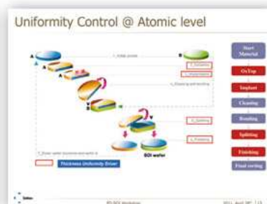
To control uniformity at the atomic level requires continual wafer-to-wafer and on-wafer control, feedback/feedforward and careful tuning of the Smart Cut process's oxidation, ion implantation, splitting and finishing steps.
