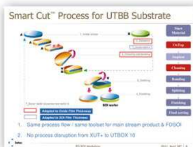
Ensuring ultra-thin silicon and BOX layers requires tuning the Smart Cut process oxidation and cleaning steps.
